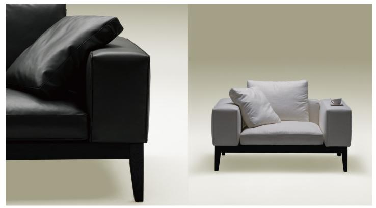
MOODIE / FRAME: Solid Birch arm and backrests covered w/fabric lined polyurethane foam. SEAT: Steel seat frame paired w/cross-woven elastic webbing & sinuous springs supporting seat cushions consisting of high-resilient polyurethane foam wrapped in feather down & polyester fiber. CUSHIONS: Back cushions filled w/feather down and polyester fiber.Toss pillow filled w/feather down. BASE: Solid Ash in Grey Oak finish. UPHOLSTERY OPTIONS: Non-removable fabric or leather.
