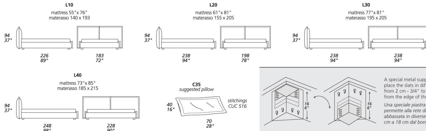
A special metal support allows to place the slats in different positions from 2 cm - 3/4" to 18 cm - 7" from the edge of the bed base.
